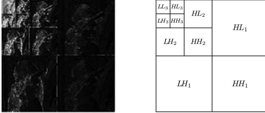
FIGURE 1. The wavelet decomposition of Lenna image with three scale levels.
