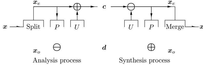
FIGURE 2. The diagram of analysis and synthesis processes by lifting scheme.
